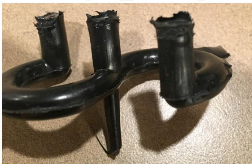
Figure 29.3 A runner with flash that will lead to flaking defects
