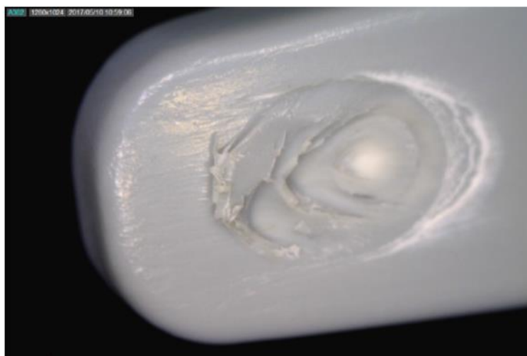
Figure 29.2 Magnified photo of sub gate with flaking
