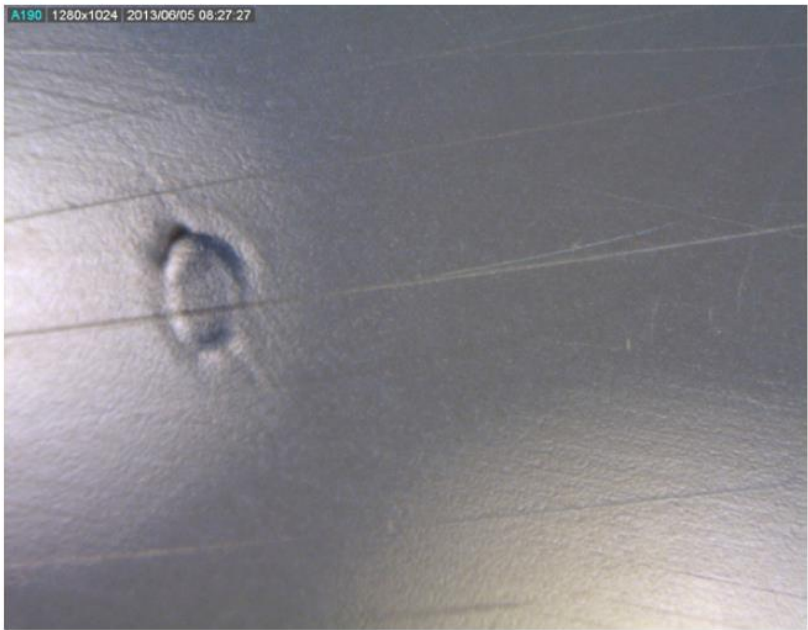
Figure 29.1 Close up photo of surface with a molded in flake
