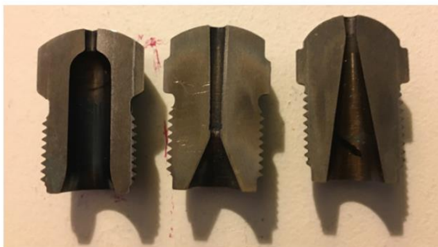
Figure 28.1 Cross section of general-purpose, nylon, and full taper nozzle tips (left to right)
