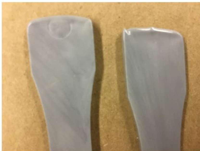
Figure 22.3 Color swirl from contamination
