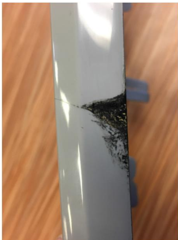
Figure 20.2 Classic example of burning from lack of venting at knit line
